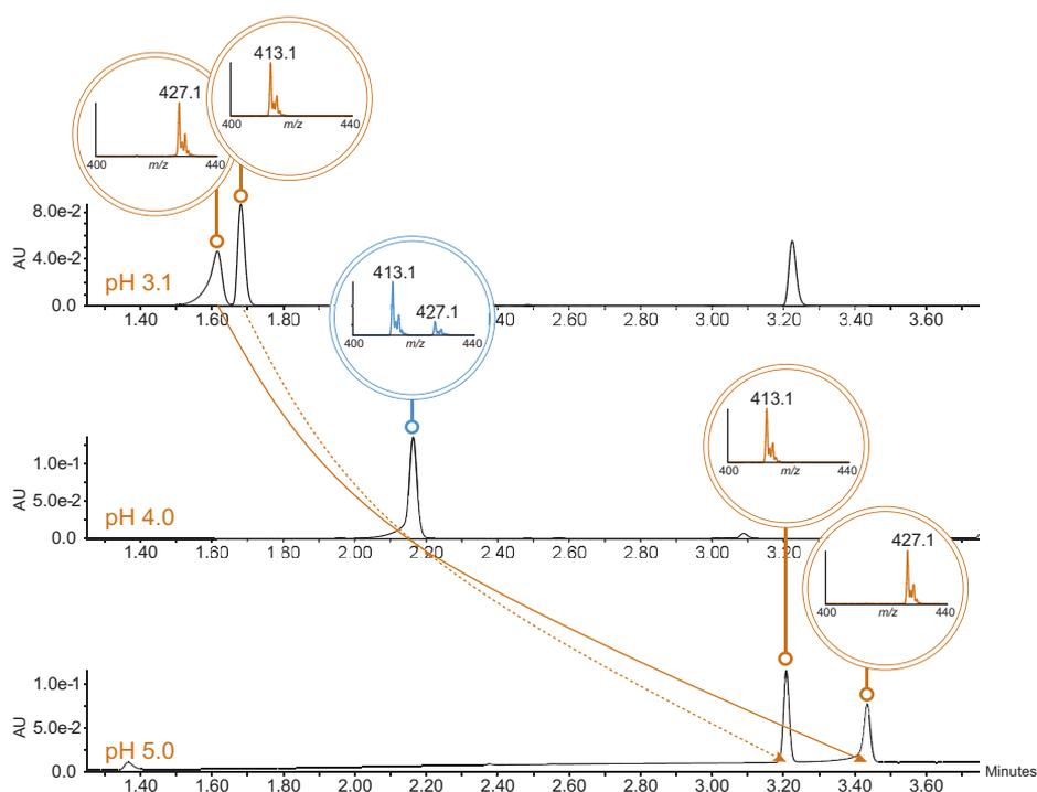
*Manipulation of chromatographic mobile phases can produce substantial and useful alterations of separation selectivity. As applied to this mixture of Ziprasidone and USP designated related substances separated with the ACQUITY UPLC H-Class System, the orthogonal selective detection available with the ACQUITY QDa Detector permits the identification of coeluting species. With changes in mobile phase, individual analytes can be tracked through changes in relative retention.*
