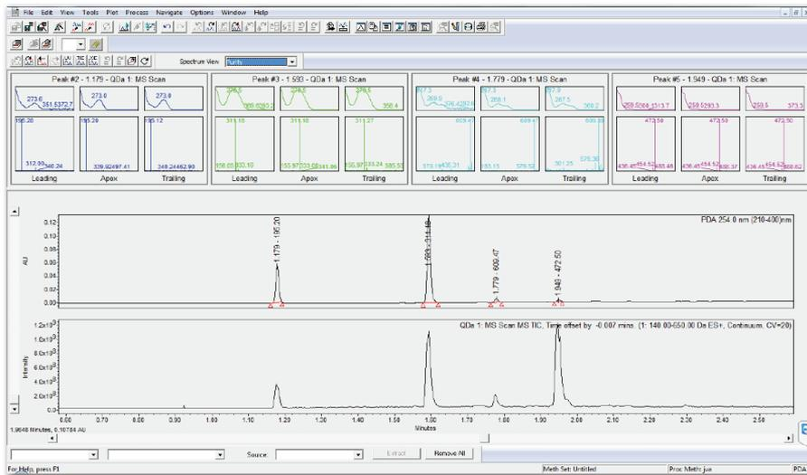
Confirm identities and highlight co-elutions in one workflow with the new Mass Analysis window in Empower 3 FR2. Chromatograms are annotated with both analyte mass and absorbance maximum, along with retention time, while the UV and mass spectra for each chromatographic peak are displayed together.
