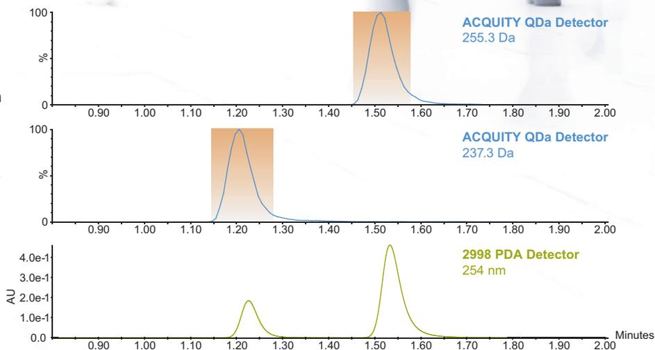
Fraction triggering by molecular mass, using the ACQUITY QDa Detector, allows selective isolation of each of the 2 components from this mixture separated using the Waters AutoPurification HPLC System.
